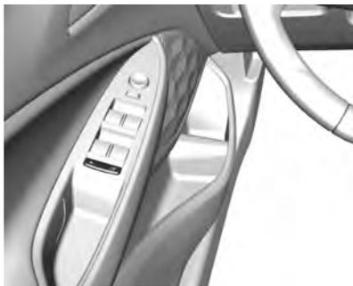
Pressione o interruptor
